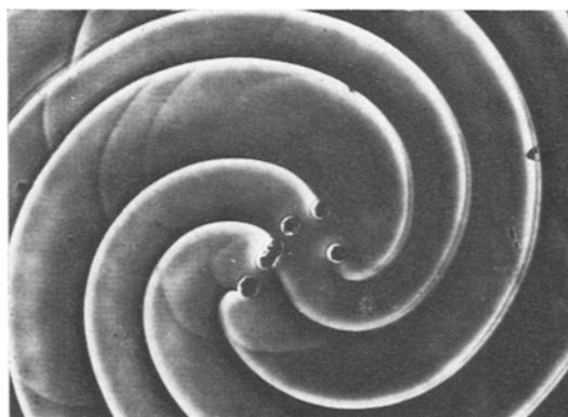
Figure 4 Positive phase-contrast micrograph of the centre of growth spirals. Etch pits were formed at the screw dislocation sites. Thin layers are also seen. ( \times 450 ).
